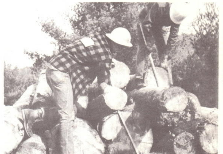
STUDENTS SCALE LOGS TO ESTIMATE THE AMOUNT OF BOARD FEET PER LOG AND TO DETERMINE THE VALUE OF THE LOG
